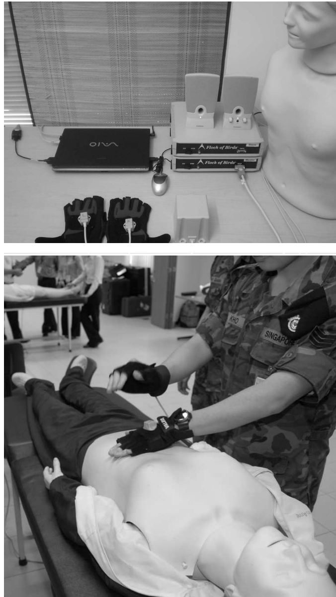
Fig. 1. Human manikin, augmented with a touch interface. The system components: the Anne Torso manikin from Laerdal Medical Corporation, Flock of Birds tracking system from Ascension, a laptop PC (1.8 GHz CPU, 1 GB RAM, Linux OS). Sports gloves are used to support motion sensors. Bottom: manikin in use. A medical student is performing physical exam by applying percussion on the manikin's abdomen.
