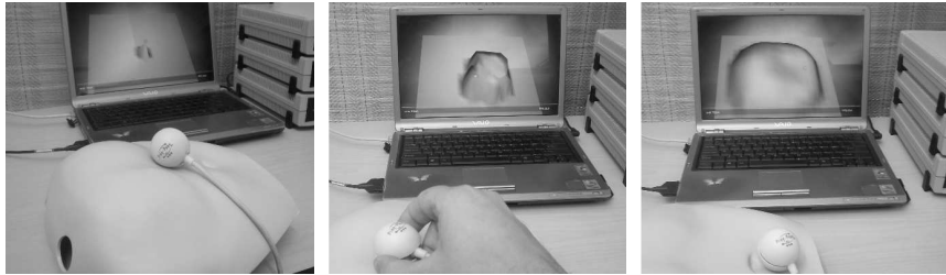
Fig. 3. Scanning SimMan's abdomen module, left to right: sensor alignment, scanning in progress, completed mesh. Grid size 40 x 40 cm, 20 x 20 points. Scanning time: less than 2 minutes.
